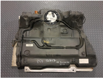
External Module and Flow Tubing Tank Fit
