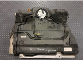
External Module and Flow Tubing Tank Fit
